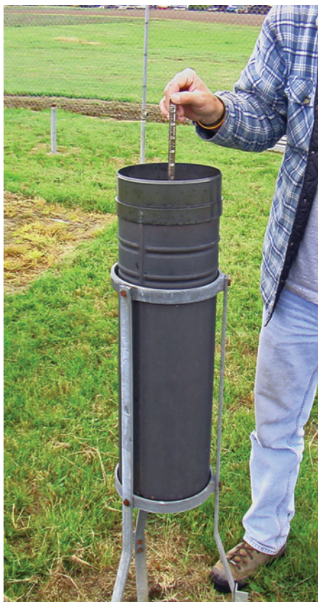
FIG. 1. Corvallis, Oregon, COOP observer Richard Mattix inserting the measuring stick into his rain gauge.
