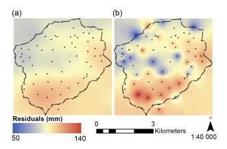
Figure 4. Residual fields of average annual precipitation interpolated with (a) ordinary spherical Kriging using 24 neighbouring stations, and (b) IDW using 12 neighbouring stations.
