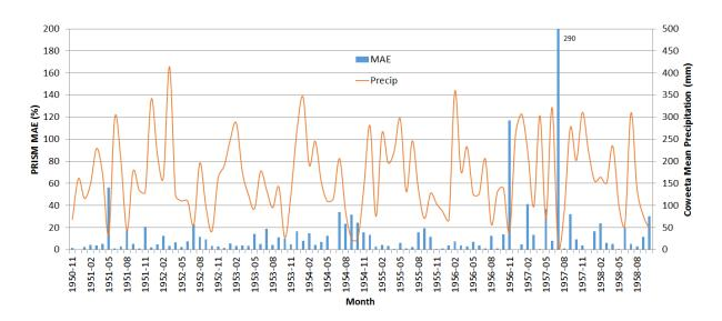
Figure S1. Time series of monthly mean absolute errors between 800m PRISM grid values and the 69 CHL stations, and average monthly precipitation for the CHL stations, over the period November 1950 – October 1958.
