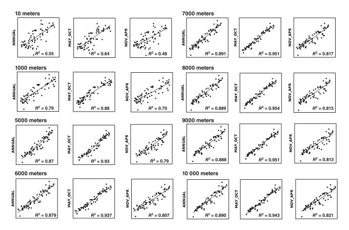
Figure 3. Scatterplots showing the relationship between the 10-m elevation grid, filtered to various wavelengths, and 1951–1958 average annual and seasonal precipitation totals at 69 stations located within the CHL.
