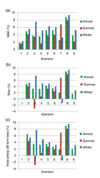
Figure 10. Uncertainty scenarios and associated error statistics: (a) MAE, (b), bias, and (c) average precipitation over the Coweeta basin. MAE and bias were determined by averaging prediction-minus-observation differences over the original 69-station dataset. See Table 5 and text for scenario descriptions.
